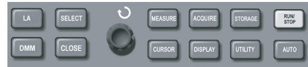
Figure 2-23 Function key for the sampling system (storage)
