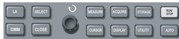
Figure 2-24 Function key for the sampling system (function) Press the [UTILITY] button to pop up the setup menu for utility functions. See Table 2-19.
