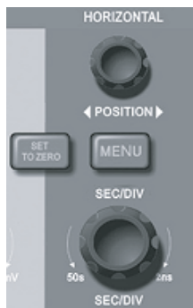
Figure 2-11 Horizontal system control interface
