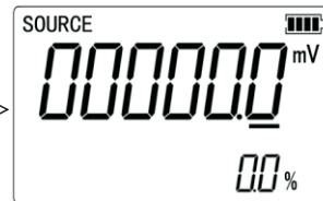
Picture 1.1-6 Voltage output 1000mV
