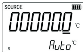
Picture 3.2-1 Auto cold junction temperature compensation
