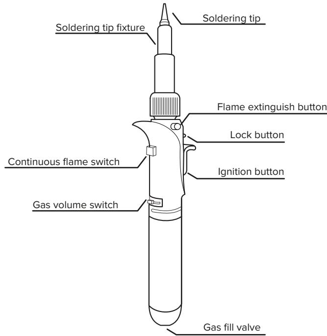
2. Press and hold the lock button, then press the ignition button.
